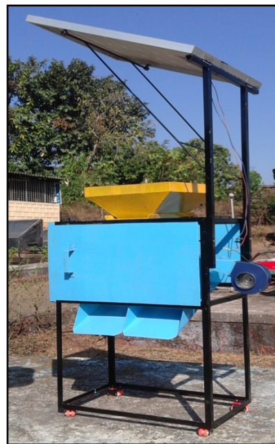
Figure 2. Pictorial view of Solar photovoltaic operated paddy winnower
