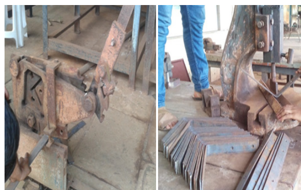
Fig. 1 Preparation of M. S. clamps: (a) cutting of M. S. strips (b) making of angles for joints (Photos@ Jain S.K.)
